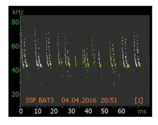
The sonogram is a presentation of ultrasound events in a chronological order. With default setting (see page 24) the frequency axis goes from 15 to 150 kHz, the time axis from 0 to 60 ms.
